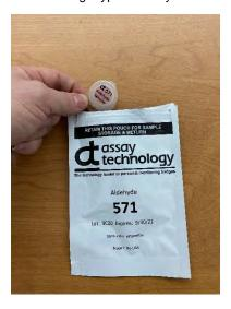
Perform your sampling by opening the ChemDisk design. Record on your chain of custody the sampling duration in minutes (or the start/stop times) for each sample. Place back in the pouch when completed.
