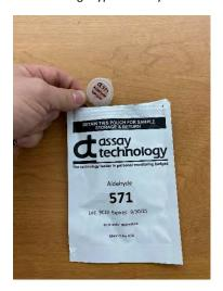
Perform your sampling by opening the ChemDisk design. Record on your chain of custody the sampling duration in minutes (or the start/stop time) for each sample. Place badge back in pouch, when completed.
