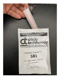
Perform your sampling by sliding the badge out of its hard-plastic case. Record on your chain of custody the sampling duration in minutes (or the start/stop time) for each sample. Place badge back in the hard plastic case, and then in the pouch when sampling is completed.
