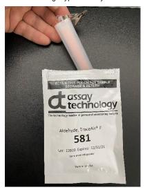
Perform your sampling by sliding the badge out of its case. Record on your chain of custody the sampling duration in minutes (or the start/stop times) for each sample. Put the badge back in its case, and then place back in the pouch when completed.
