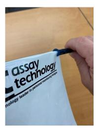
If fed correctly, you can pull the Seal Stick over the rest of the pouch. Place one of the provided information labels on the pouch, your badge is now ready for shipment. Do not utilize any sort of tape, as that may invalidate your sample.
