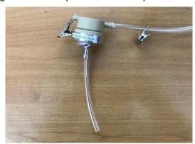
2) The tubing connected to the calibration adapter connects to the calibration device. The outlet of the PPI (from which the black cover was removed) will be connected to the pump tubing. Allow the pump to warm up for at least 1.5 minutes to achieve a true flow.
