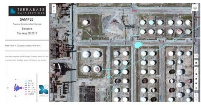
Example: AIHR Sharks surround the perimeter of the potential sources. Through vectoring, the emission source can be tracked prior to or post exceedance of a benzene "hit" on a TD Tube.
