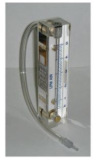
The formula on the side of the rotameter was developed after calibration with a Dry-Cal. Use this formula, the temperature, and pressure to determine the actual flow rate at the sampling site *prior to sampling*.
