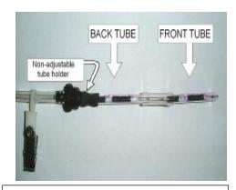
When sampling with two tubes in series, make sure the direction of air flow is still from front to back
