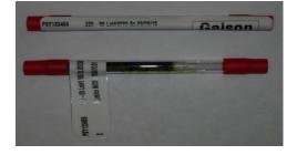
Preferred sampling tube labeling. **DO NOT** utilize tape or any other adhesive to seal tubes, seal sample by placing red caps on ends. Anything other than shown above may contaminate sample.
