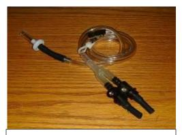
Dual splitter for multiple sampling. Please try to avoid adjusting flow rates with this equipment
