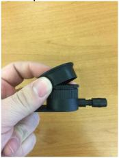
Warning: Twisting the cap will cause the IOM to come apart and potentially impact the IOM integrity.
