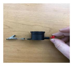
4) Connect the DIS to the pump via the provided tubing and turn the pump on to begin event.
