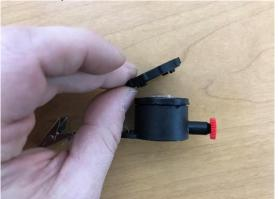
Warning: Twisting the cap will cause the DIS to come apart and potentially impact the DIS integrity.
