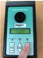
3) Place the Air-O-Cell cassette on the inlet of the pump, with the arrow pointing down.
