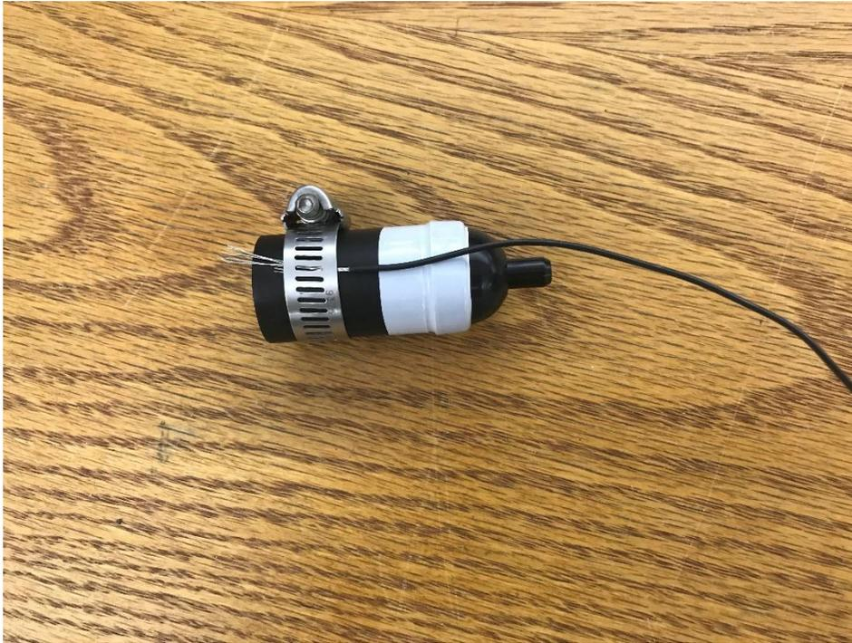
When sampling for Asbestos in this fashion, it is recommended that you ground your cassette to remove the possibility of static during your sampling event. SGS Galson has provided a clamp and a stripped grounding wire for this use (**both must return to SGS**).
