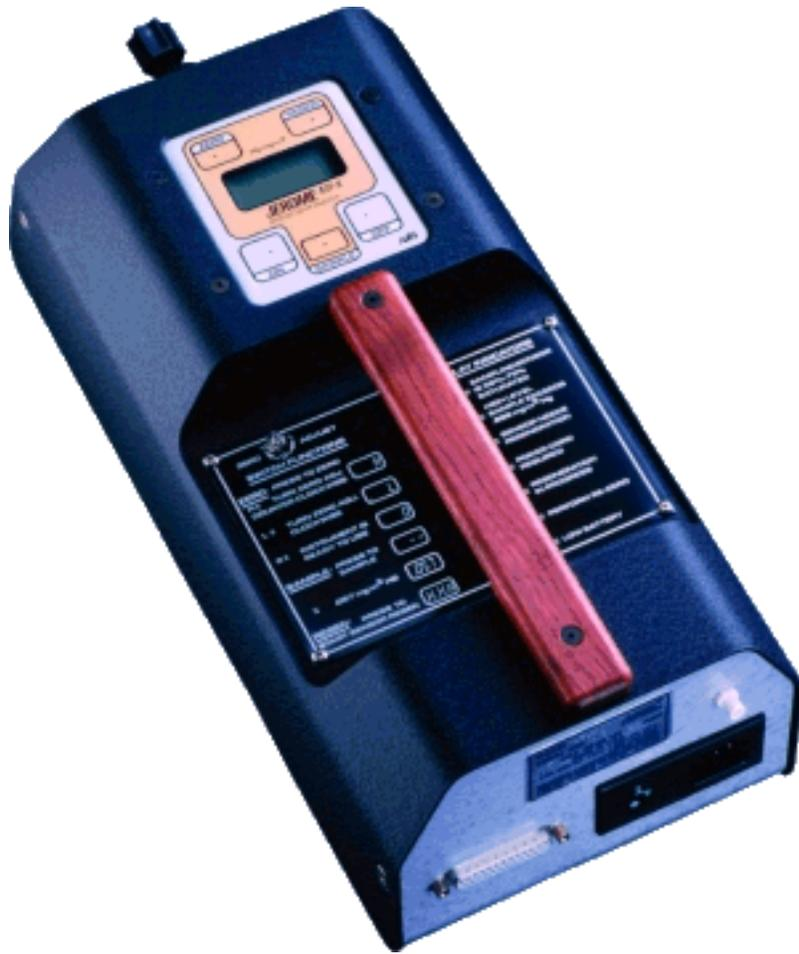
The Jerome 431-X mercury vapor analyzer uses a patented gold film sensor for accurate detection and measurement of toxic mercury vapor in the air. This portable hand-held unit can easily be carried to locations with mercury concerns for applications such as industrial hygiene monitoring, mercury spill clean up and mercury exclusion testing. Simple, push-button operation allows users to measure mercury levels from 0.003 to 0.999 mg/m<sup>3</sup> in just seconds.
